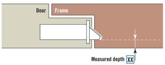
To find the right striker for your application, measure the distance from the door face to the edge of the springbolt of the latch.
